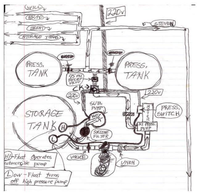
Well drawing - this was a joint effort between Chalon and Brenton to figure out the control system for the irrigation and residential water supply. A lot of head scratching went into this design, which both Chalon and Brenton agree they couldn't have figured out on their own. The system has worked great so far.
